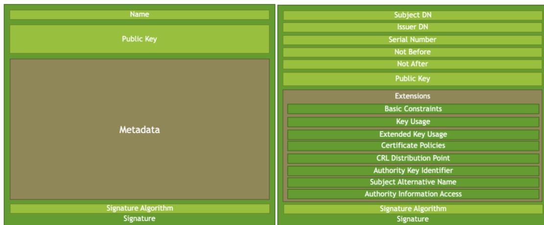
Figures 1 and 2: Key components of a PKI certificate that support identity including Name, key, metadata, signature algorithm, and signature. Additionally, a detailed listing of several possible elements of a PKI certificate.
